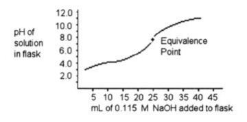
25) A 50.0 mL sample of a solution of a monoprotic acid is titrated with a 0.115 M NaOH solution. The titration<br/>curve above was obtained. The concentration of the monoprotic acid is about \_\_\_\_\_ mol/L.<br/>A) 0.120 B) 0.0600 C) 0.240 D) 25.0 E) 0.100<br/>Answer: B
